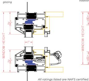
Shown with narrow sightline, nailing fin and traditional, sloped exterior glazing
