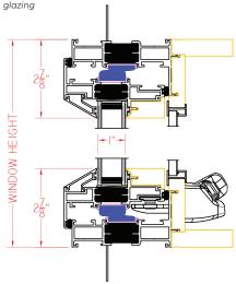
Shown with nailing fin and traditional, sloped exterior
