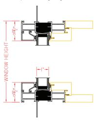
Shown with nailing fin and traditional, sloped exterior
